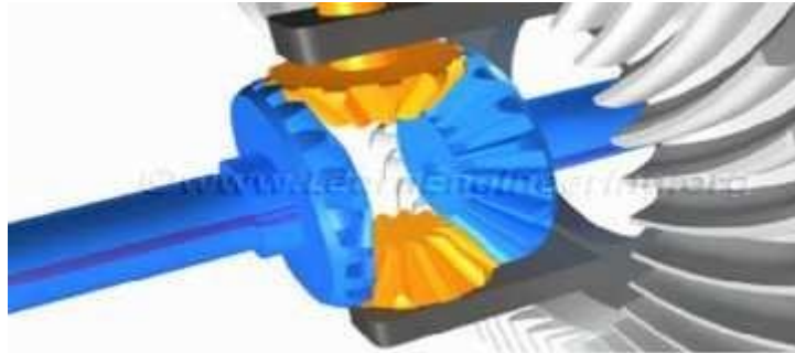
Double spider gear arrangement
