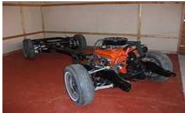
Rolling X-frame chassis
