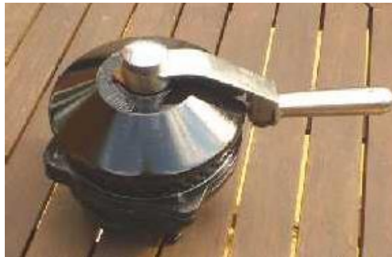
A driver's brake valve for a DMU. Photo: Traction ads.
