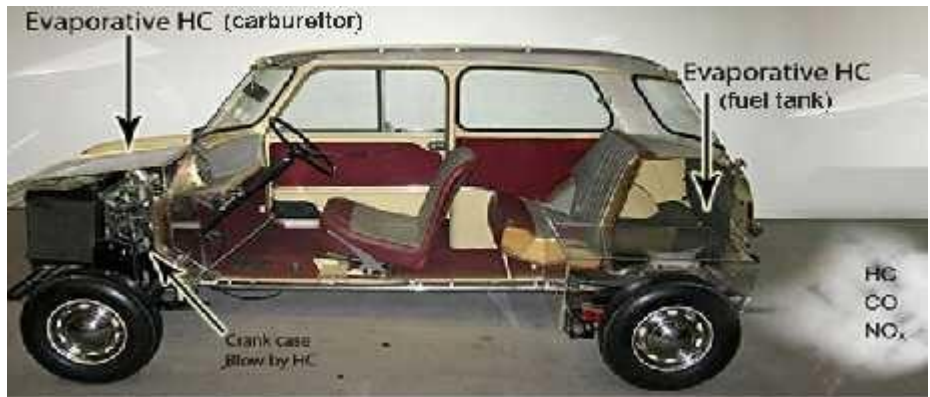
Emission sources in a gasoline fuelled car.
