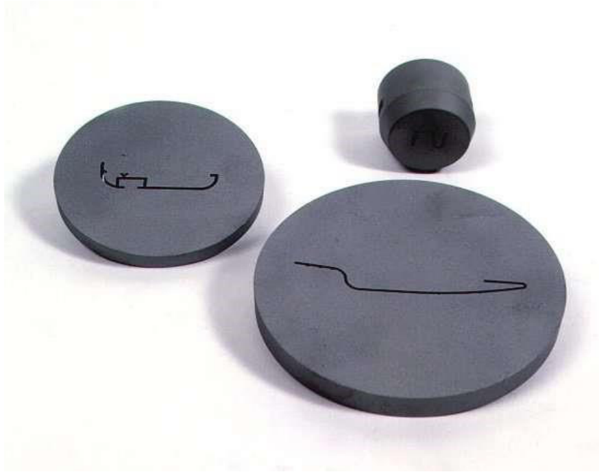
Figure 16: Sparked eroded extrusion dies
