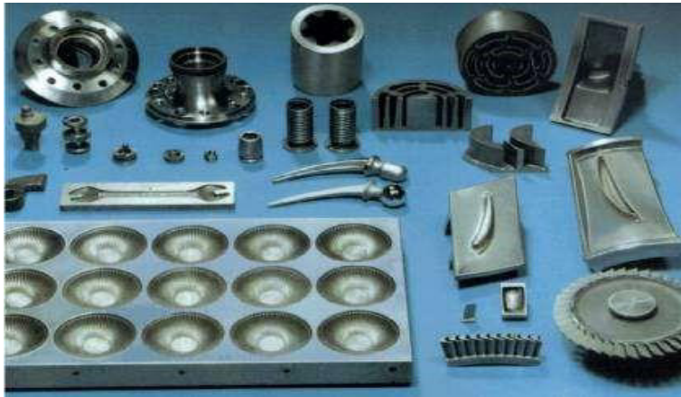
Figure 9: Parts made by ECM
