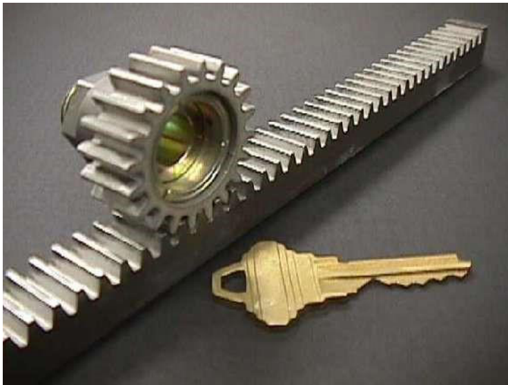
Figure 6: Steel gear and rack cut with an abrasive water jet
