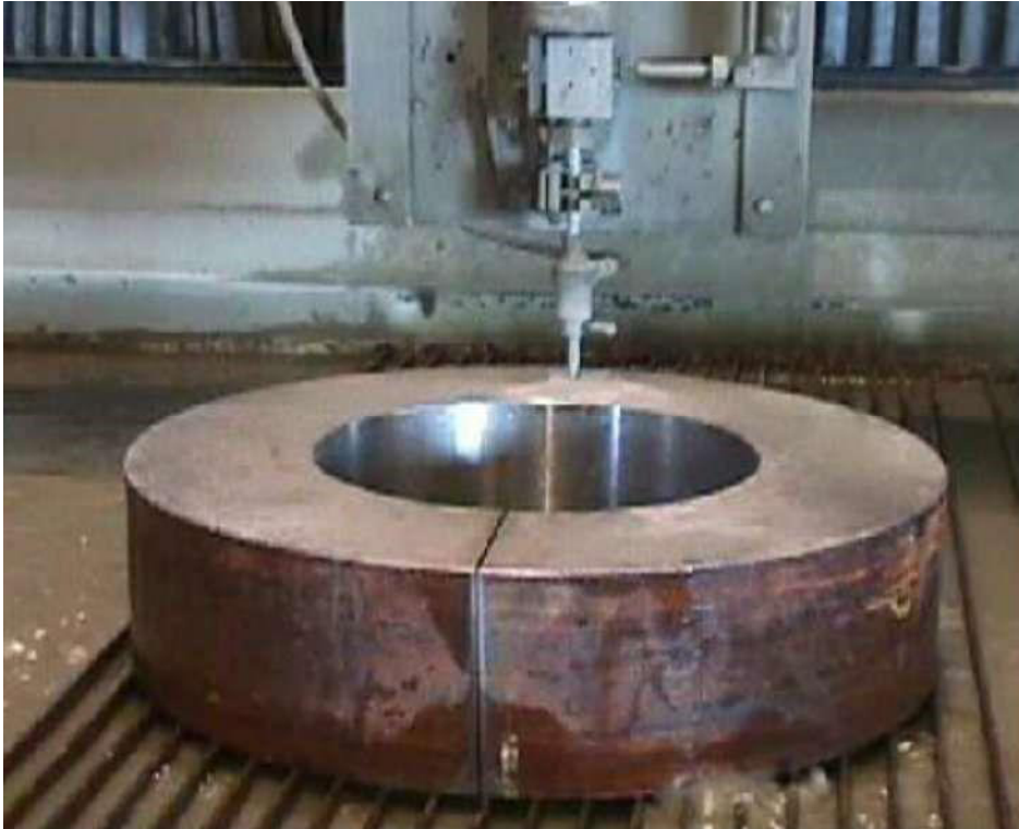
Figure 5: Abrasive water jet cutting
